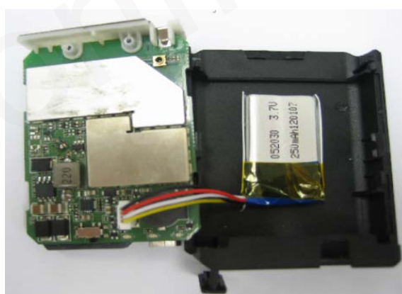
Figure 6. Backup Battery Installation
