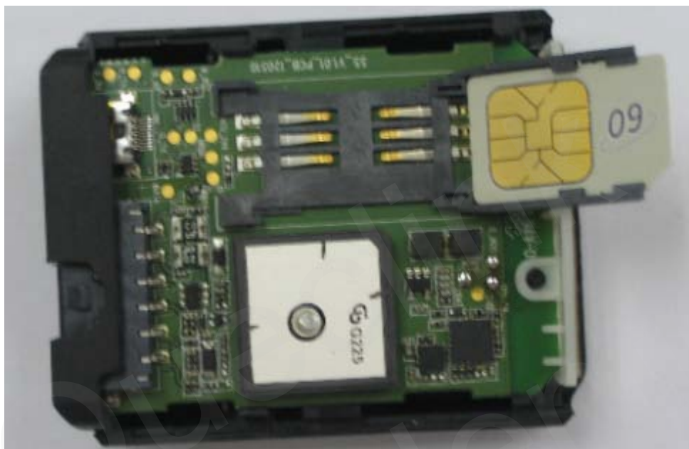
Figure 5. SIM Card Installation
