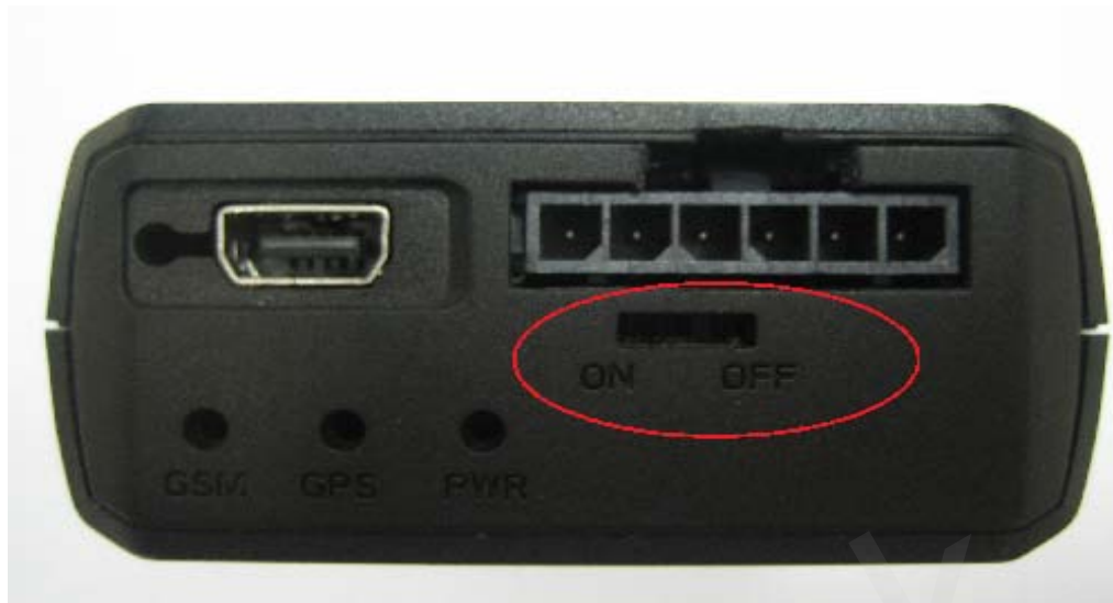
Figure 7. Switch and ON/OFF position
