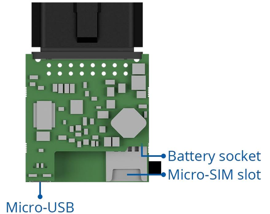
Figure 1 FMB001 device view
