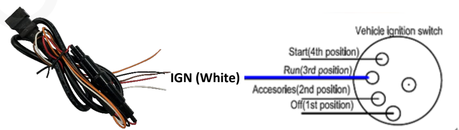
Figure 4. Typical Ignition Detection
