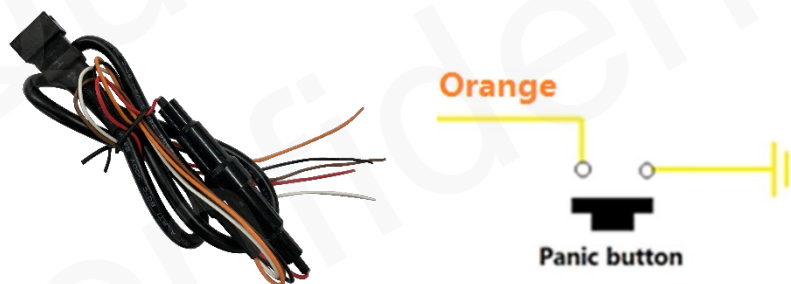
Figure 5. Typical Digital Input Connection
