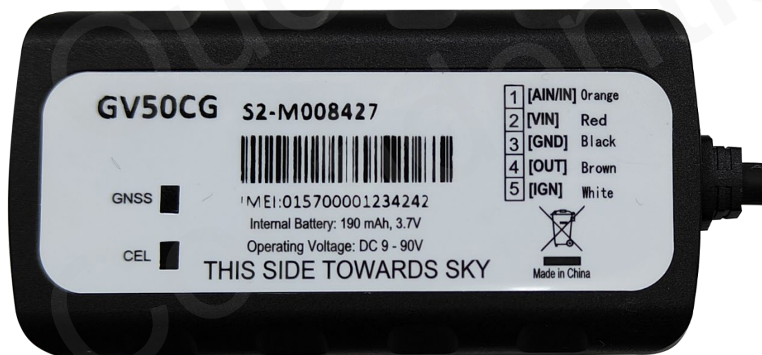
Figure 8. GV50CG LEDs on the Case
